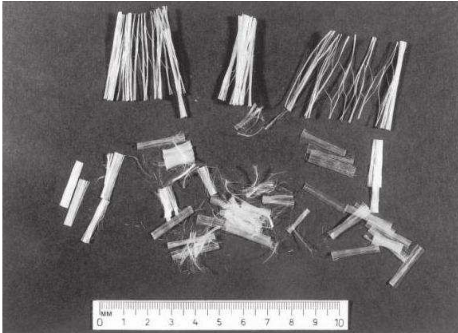
Figure 5.1.: Types of polypropylene fibres (PPF).
