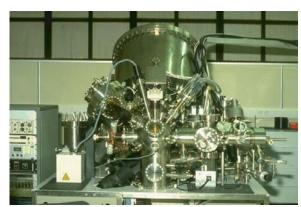
**Figure 2-1: (a)** Schematic of an XPS set up shows X-ray source for the production of X-rays and detector to measure kinetic energy and number of electrons (reproduced from (8)); (b) Photograph of Scienta ESCA 300 used in the current experiments.
