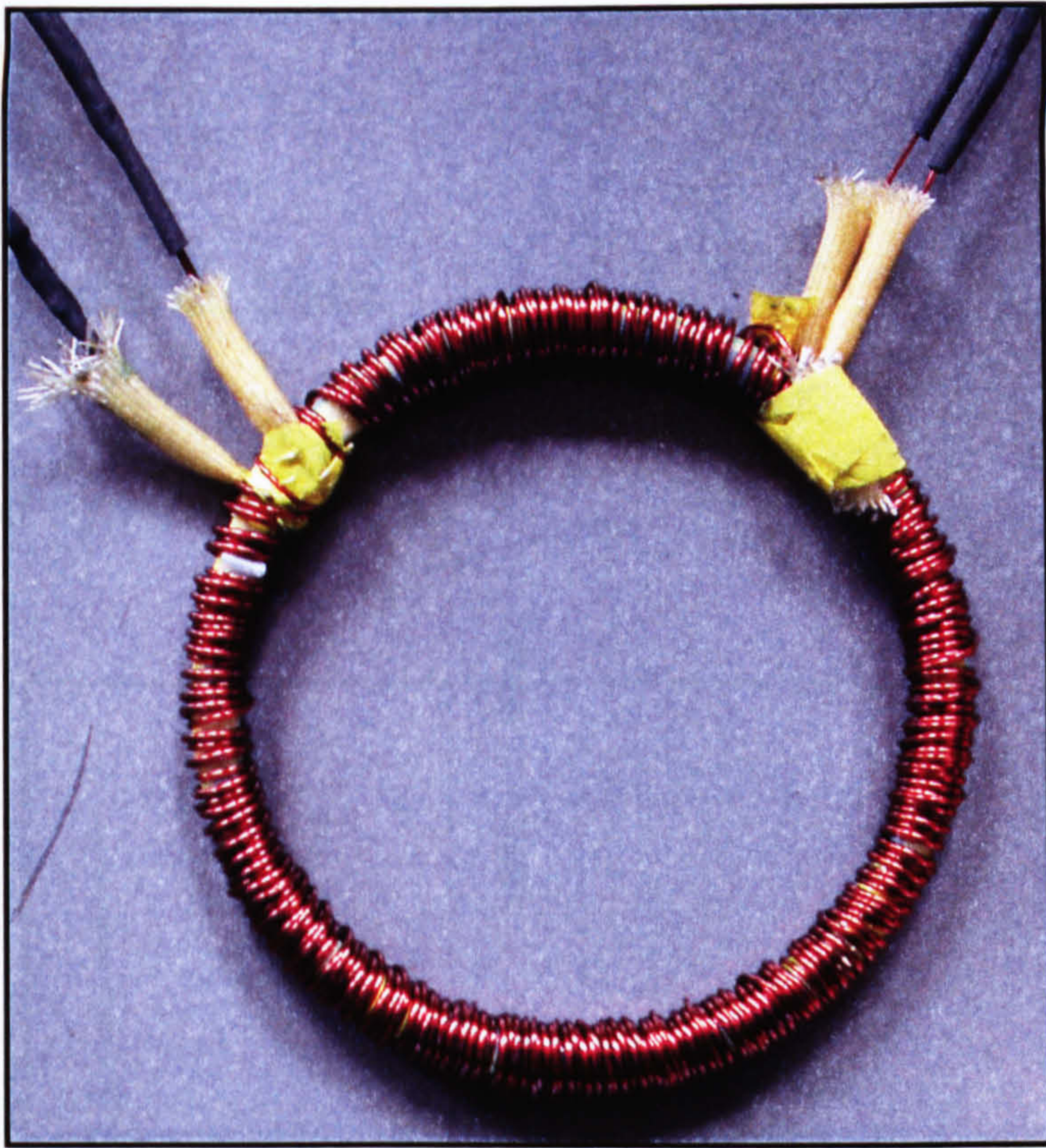
Fig. A6.5. Toroid ring sample for use in iron loss tests
