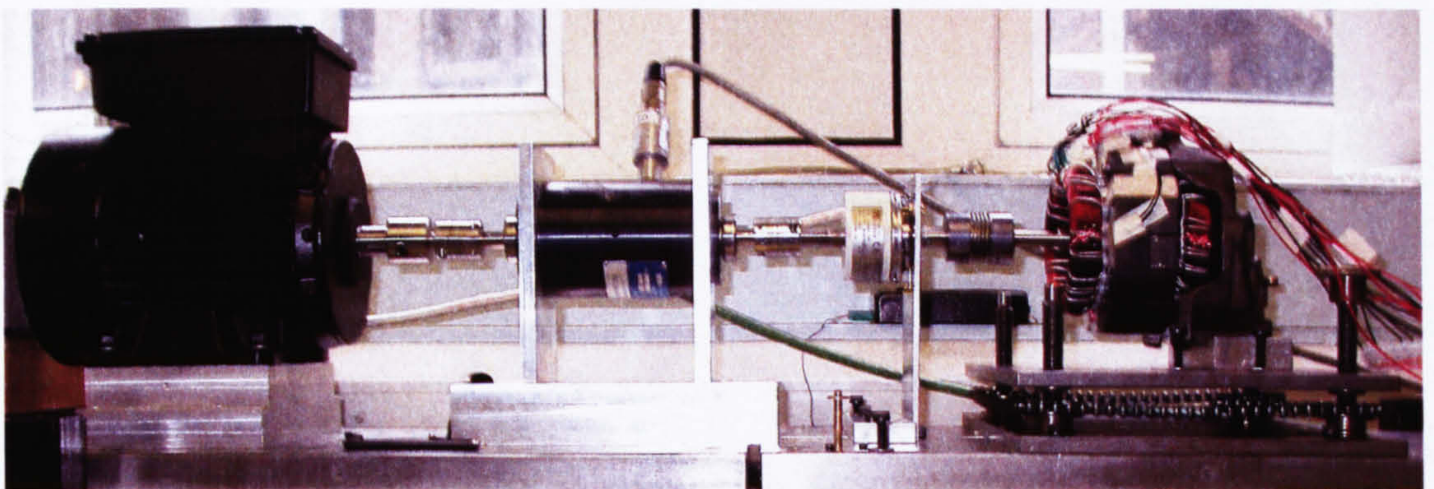
Fig. 2.3. Dynamometer test rig for magnetisation curve measurement.
