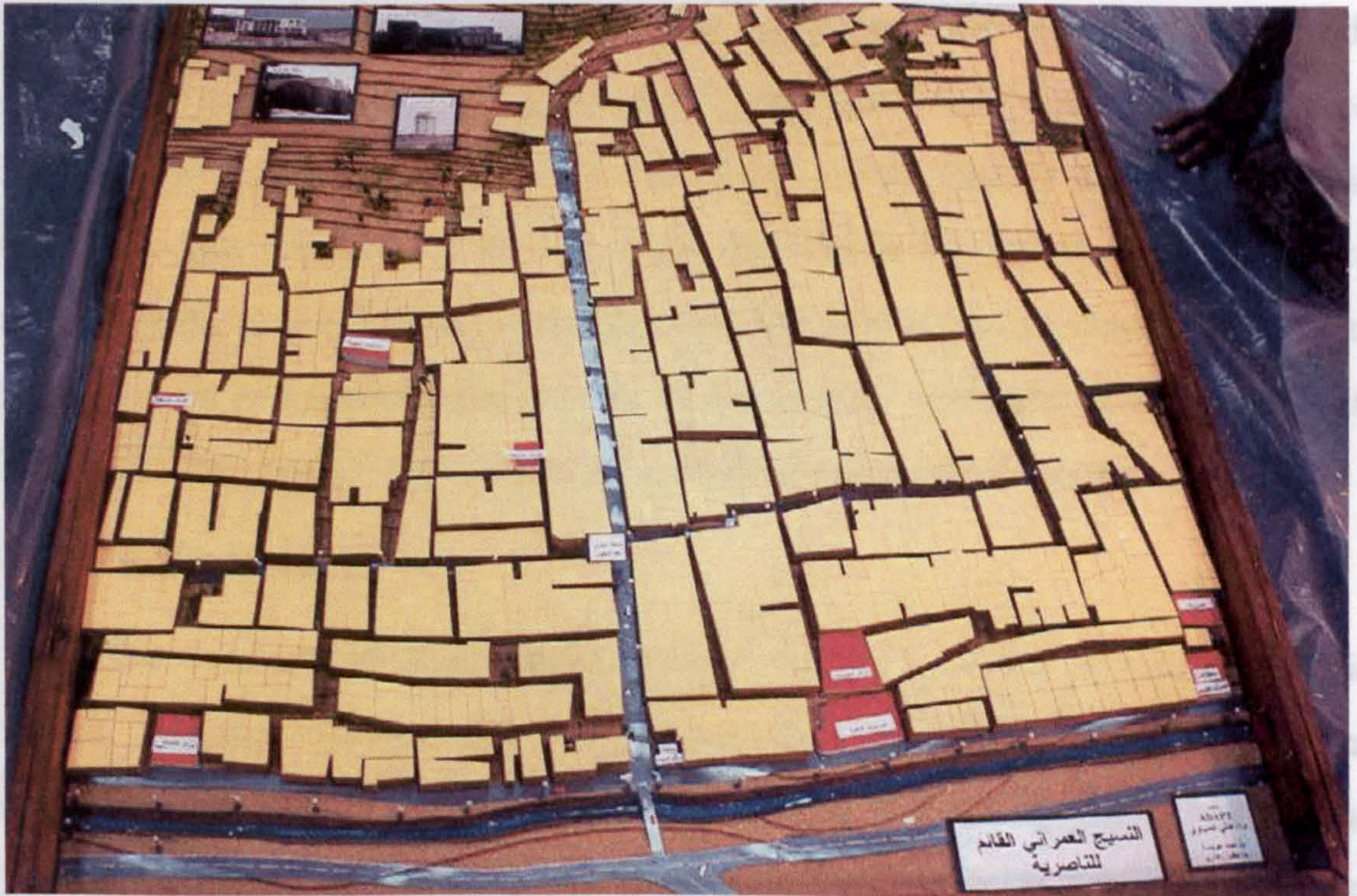
Plate 7.4: Nasriya: Land regularisation plan. Once a householder wants to re-build the house, he/she has to set the main façade back up to 1.5m (e.g. horizontal and vertical middle streets in the photo). This simple model was presented in public meetings as well as for disseminating the experience elsewhere.
