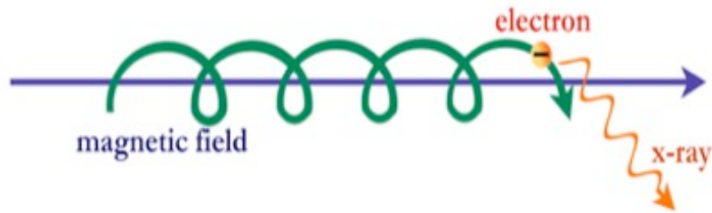
Figure 1.7: Schematic diagram showing synchrotron emission. Courtesy S. Bank, University of Wisconsin-Madison
