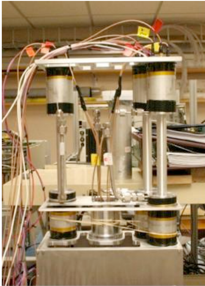
Figure 5.3: The new FNIT prototype with 3 rods, each filled with liquid plastic scintillator
