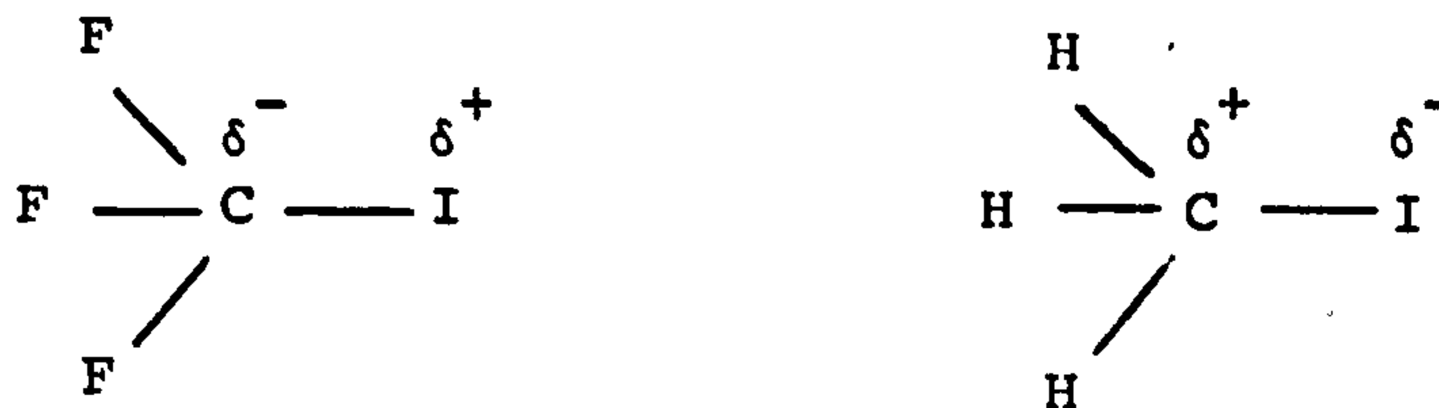
Fig. (3.14) - The presence of fluorine in a molecule changes the polarity of carbon halogen bonds.
