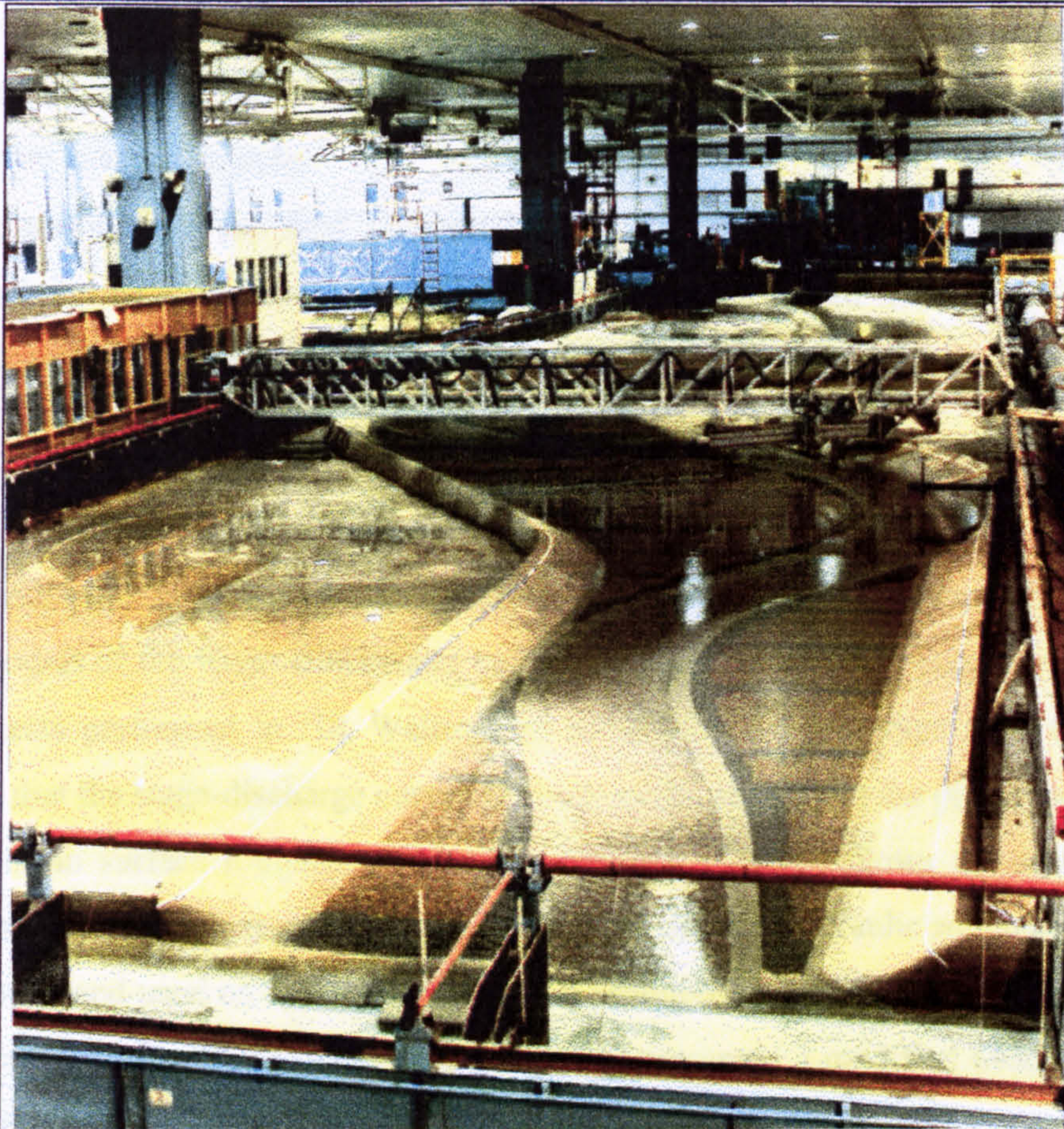
Figure 2.45 The 1:5 scale model of the River Blackwater (after NRA[1996])
