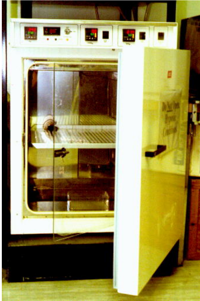
Figure 2.9: Humidified temperature controlled incubator (Model GA156; LEEC, Colwick, Nottingham, UK)
