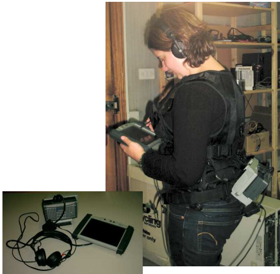
Figure 8.6: An example of how the Xybernaut device was worn by participants and (insert) the device itself.
