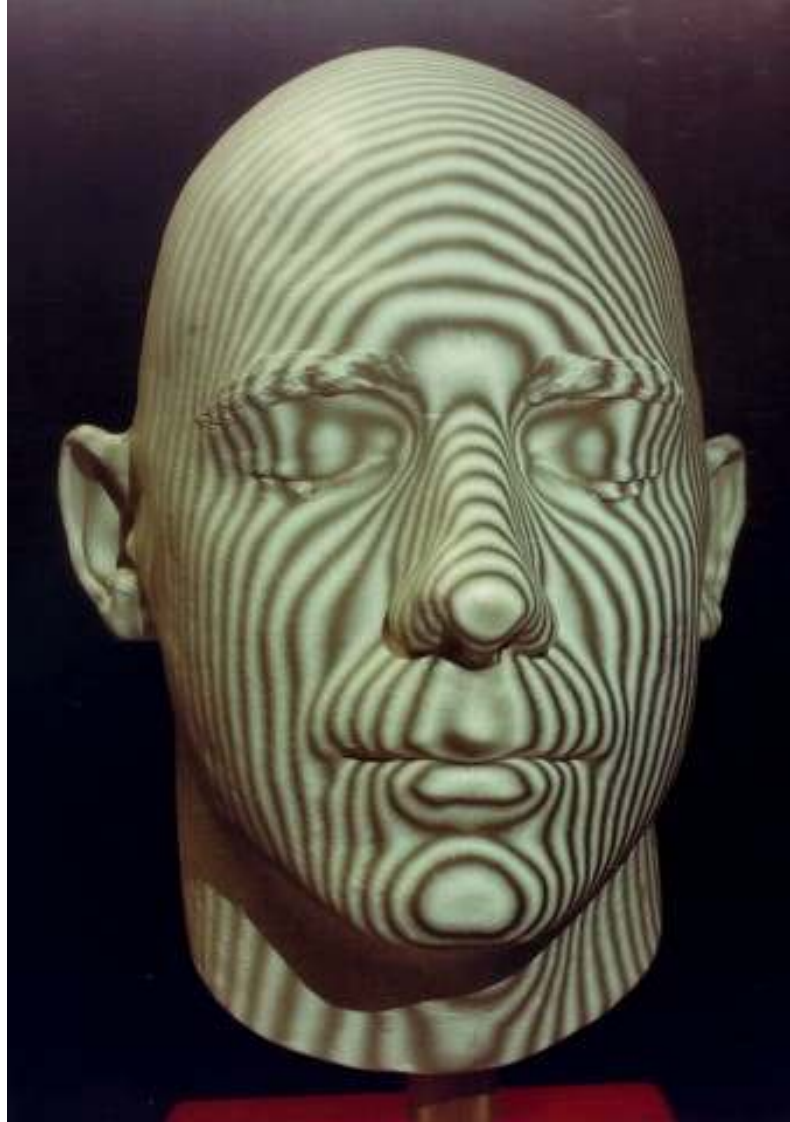
Figure 1.6 Photograph showing the image of a face captured by the technique of Moiré Topography .
