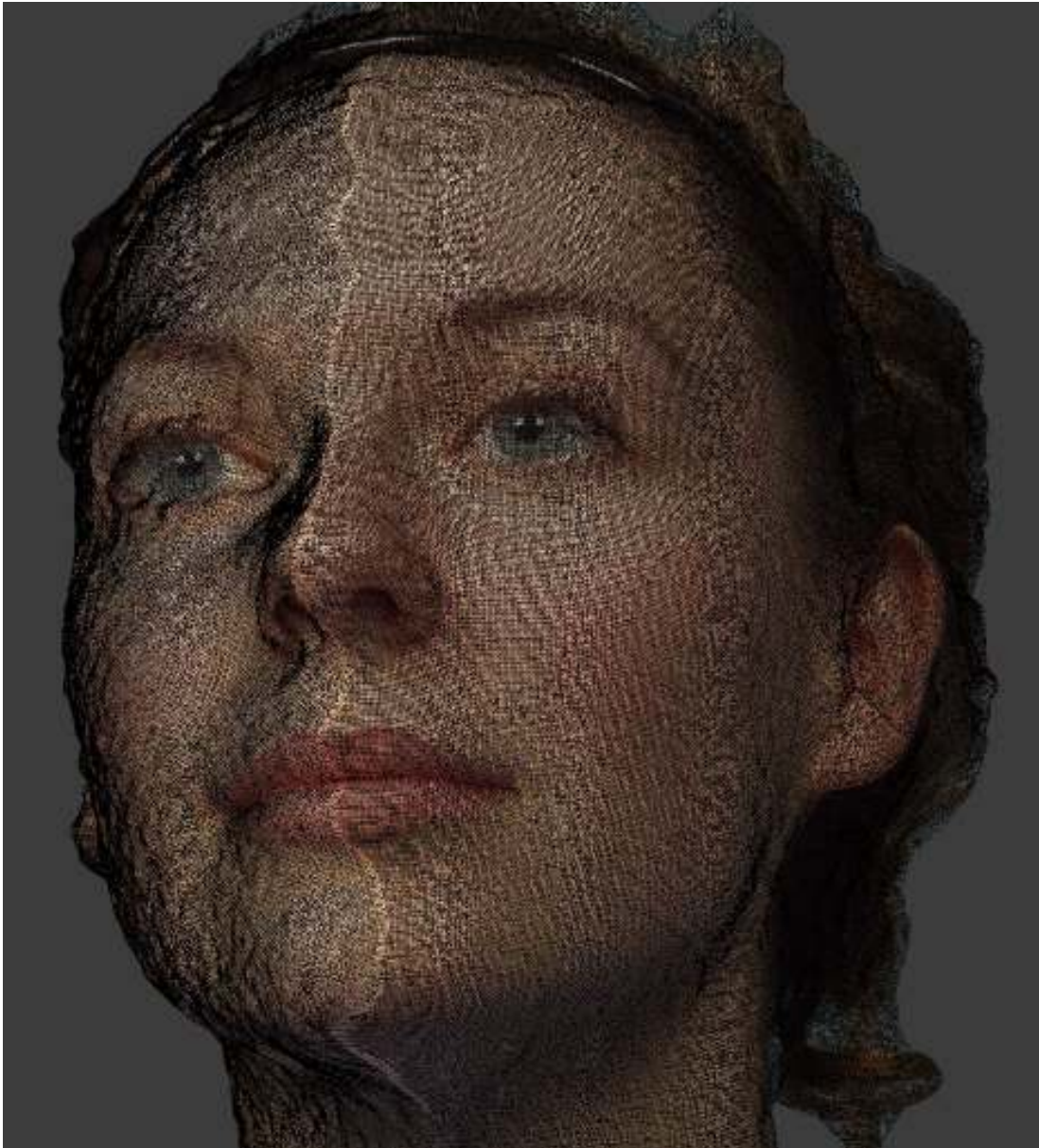
Figure 1.10 Photograph showing the image of a face captured by the Di3D system with the wire mesh overlaid to show depth and the quality of the three-dimensional model building.
