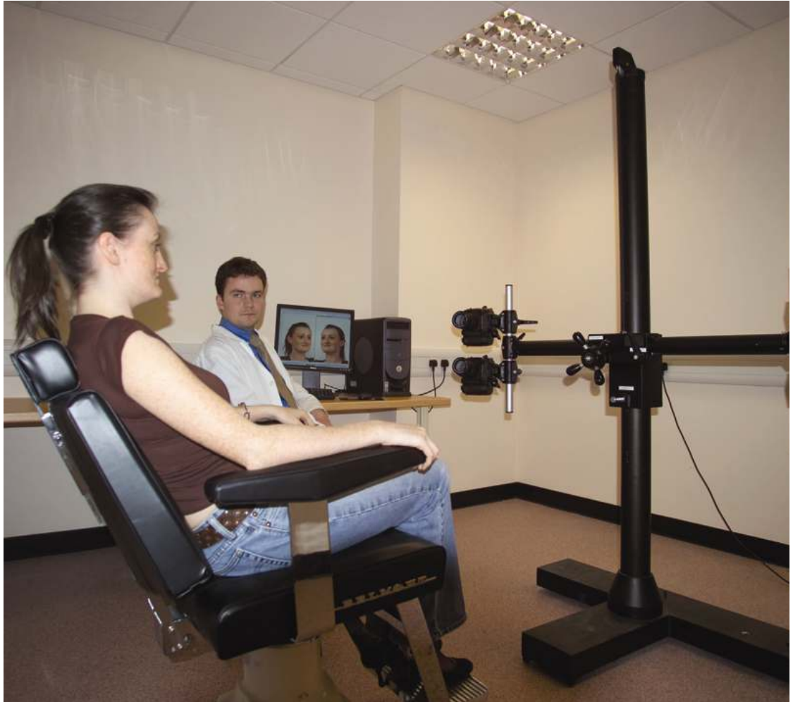
Figure 3.1 Photograph showing a subject being imaged using the Di3D stereophotogrammetry system
