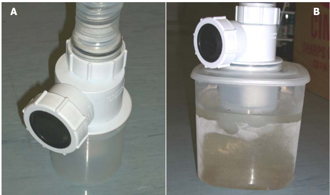
Figure 7: The condensation chamber has a one way valve (A) at the end of the system to isolate of from the environmental air. The PP chamber (B) in immersed in the ethanol/liquid nitrogen slurry
