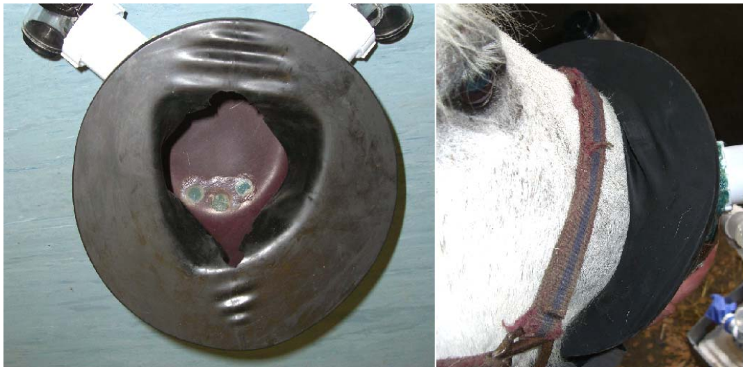
Figure 4: the rubber shroud sealed the mask on the muzzle of the horse creating a closed unidirectional circuit preventing contamination of the exhaled breath sample with ambient air and permitting generation of negative pressures necessary to activate the one-way valves.
