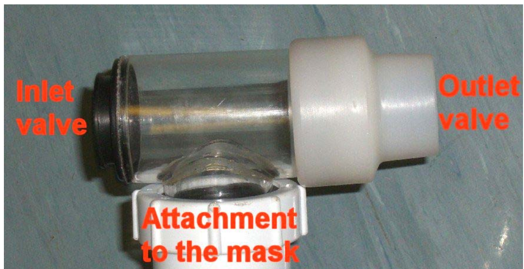
Figure 5: One-way valves used in the study. Two valves were connected to the mask. Each valve has an internal diameter of 3.5cm and ensure a unidirectional flow of air during respiration by the horse
