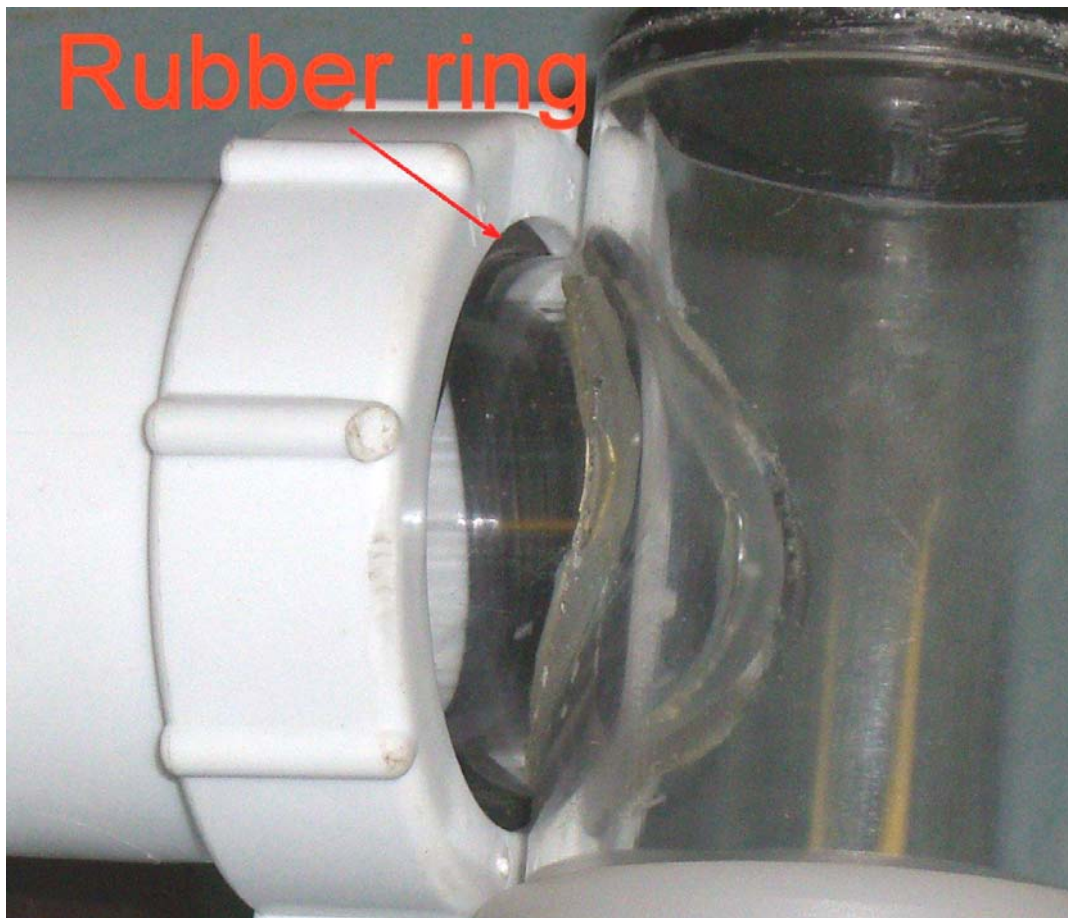
Figure 3: A rubber ring was used to establish an air-tight connection between each one-way valve and the mask
