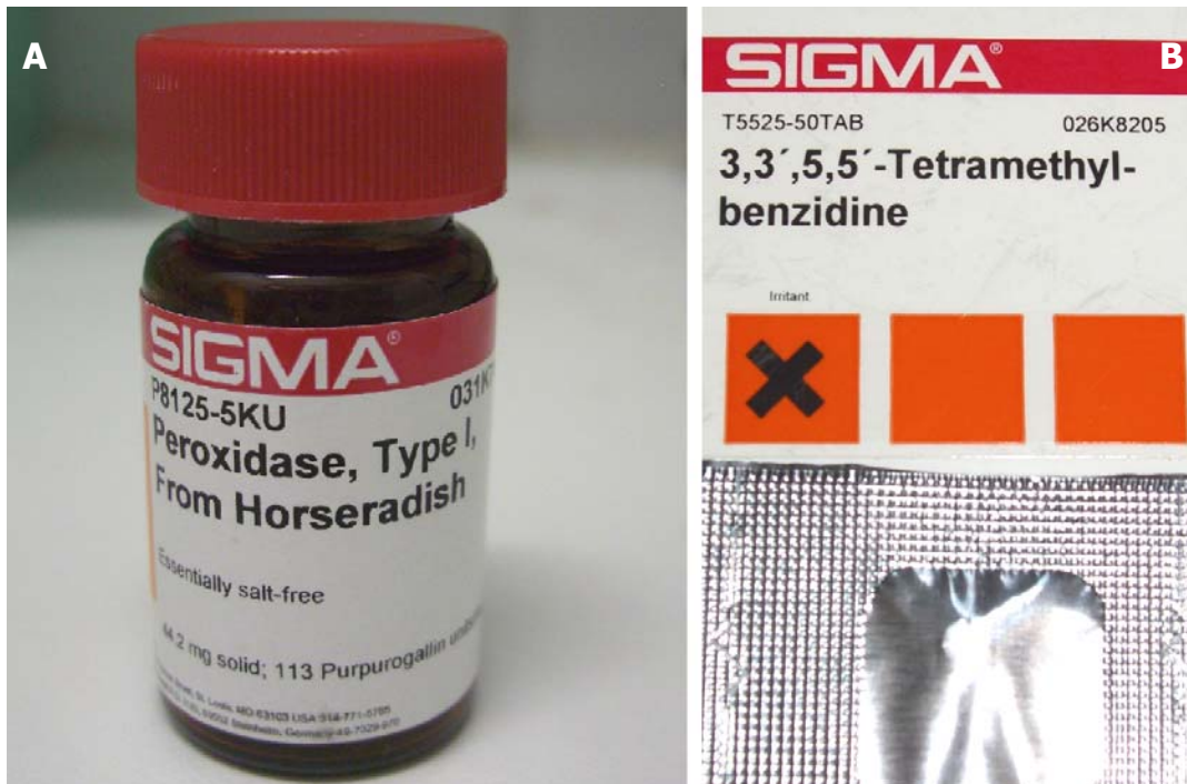
Figure 1: A) The Horse Radish Peroxidase (HRP) was available as a powder and was reconstituted as a solution by adding 1.36ml of distilled water for every mg of powder; B) The TMB (3,3',5,5'-tetramethylbenzidine) used was available in 1mg tablets and was prepared in solution mixing 1mg of TMB with 0.5ml of Acetone, 0.5ml of methanol and 9ml of 0.42M citrate buffer solution (pH 3.84)
