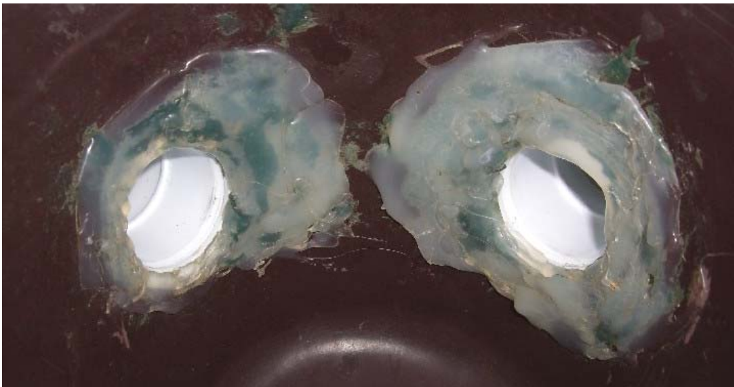
Figure 2: inner view of the mask where two holes were left open and modelled with fibreglass and artificial resin to fit the attachment of the one-way valves
