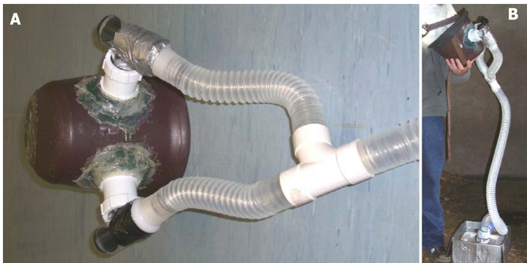
Figure 6: A) The connection of the face mask to the condensation chamber was obtained through flexible rubber/plastic tubes; B) The device is used in the standing non-sedated horse
