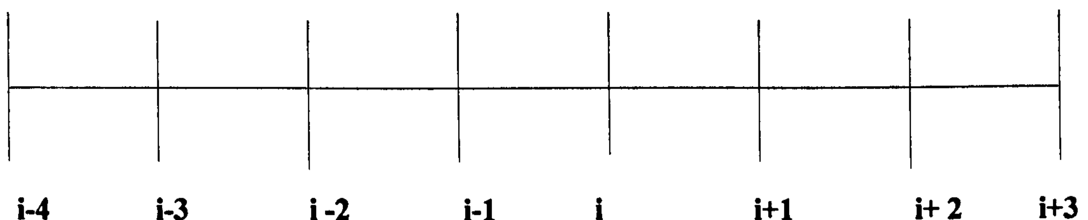
Figure (4.3) One-Dimensional Grid used for the derivation of the 8 Point Method of Characteristics
