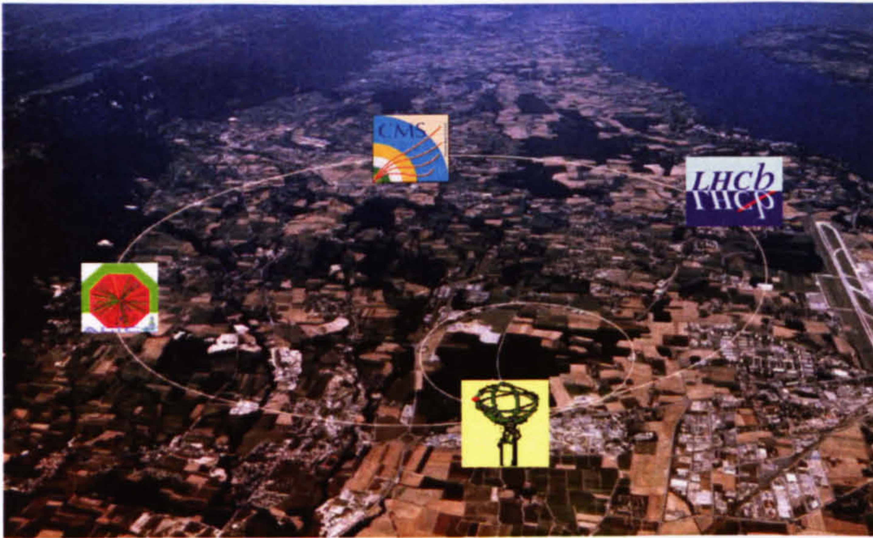
Figure 2.1: Aerial view of the CERN and the surrounding region. The largest ring is the LHC that has a circumference of 27km. The approximate locations of the ATLAS, ALICE, CMS and LHCb experiments are also highlighted. This figure is modified and reproduced from [80].
