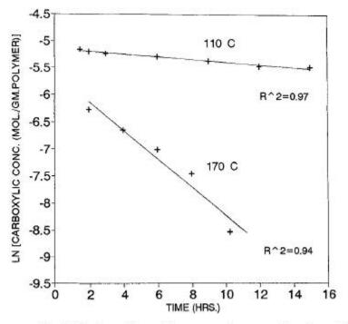
Fig. 5 Carboxylic acid conversion as a funcion of time and reation temparature.
