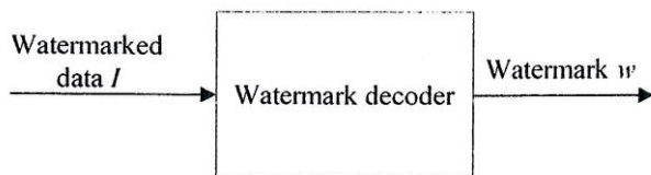
Figure 1. Multi-bit watermark extraction system
