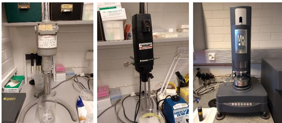
Figure 23. The equipment used for mixing of suspensions and rheometer. Left: Omni Mixer Sorvall, middle: Heidolph Diax 600, right: Texas Instruments AR-G2 rheometer.
