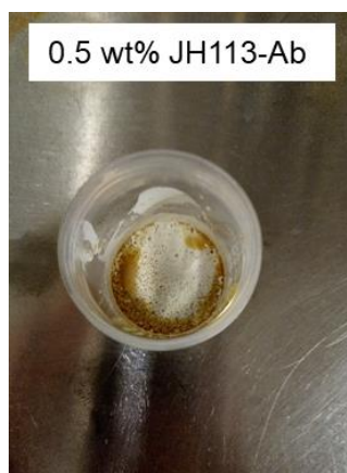
Figure 30. Suspension with 75 % \text{TiO}_2 and 0.5 wt% JH113-Ab of \text{TiO}_2 after storing of 7 days and before remixing.
