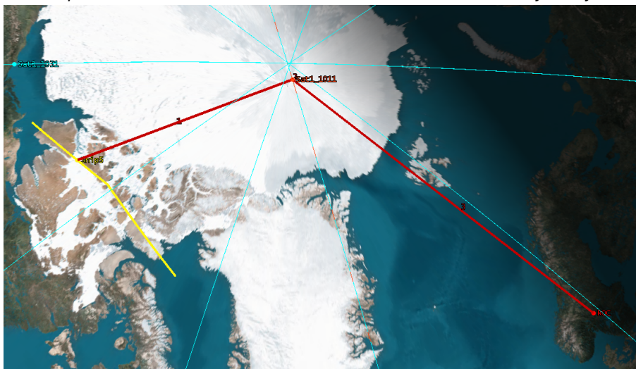
(b) Multi-hop link at 1000 km altitude vessel-GW without ISL and one-way delay of 21 ms.
