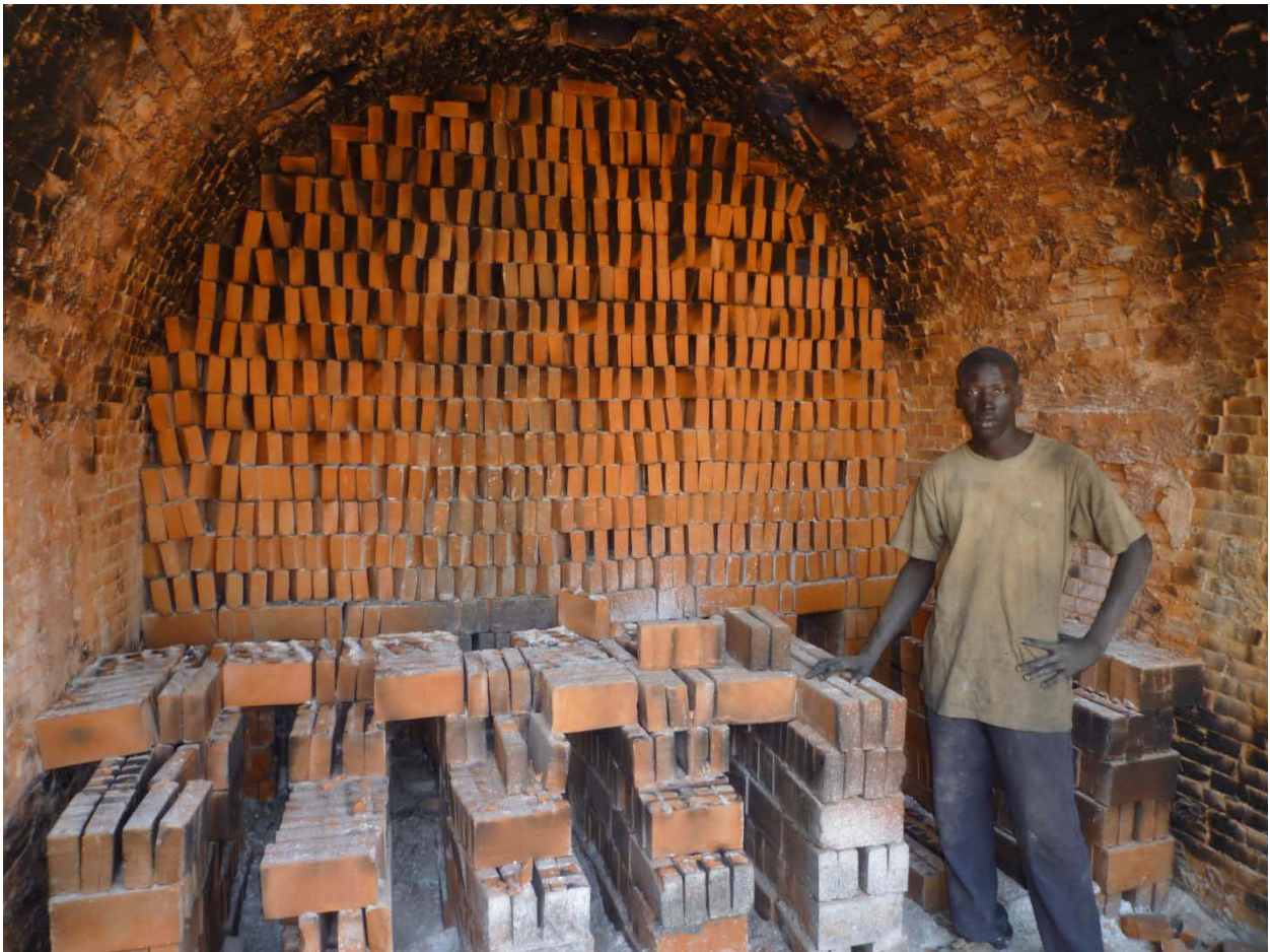
Figure 2. Tunnel kiln, Marisa Brick Company, The Gambia
