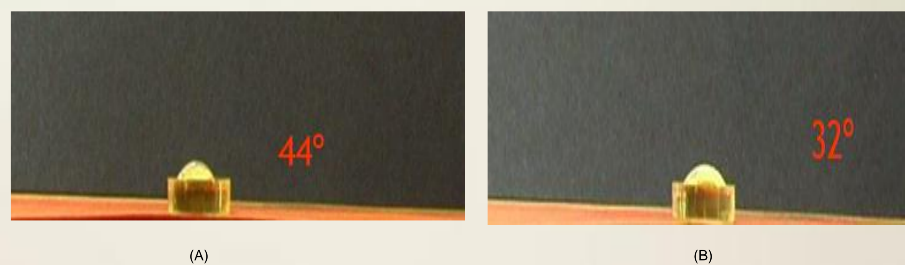
Fig 5: Diagram to show contact angle of Gamma sterilised PMMA after one day immersion in Buffer, measured as 44° (A) and Contact angle of Gamma sterilised PMMA after 9 weeks immersion in Buffer, measured as 32° (B)
