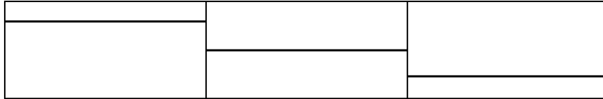
First order method: Flow variables are treated as constant across a cell.
