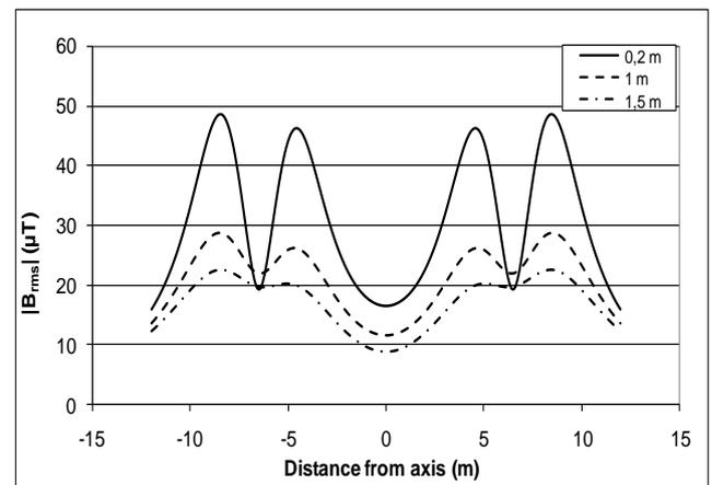
Fig. 5. Distribution of magnetic flux density for normal operation
