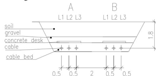
Fig. 1. The cable distribution in the trench
