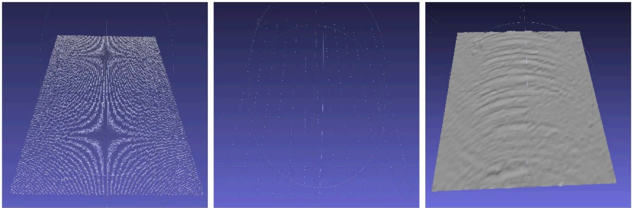
Figure 5: Three-dimensional point cloud associated with the profile of a steel tool surface (a), the extracted boundary curves (b) and the resulting PDE-based surface representation (c).
