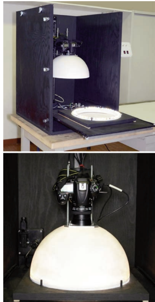
Figure 1. The Computer Vision System (without front and top walls) in which camera and the white hemisphere are lifted up to allow samples arrangement (on left); the same system during image acquisition (on right).
