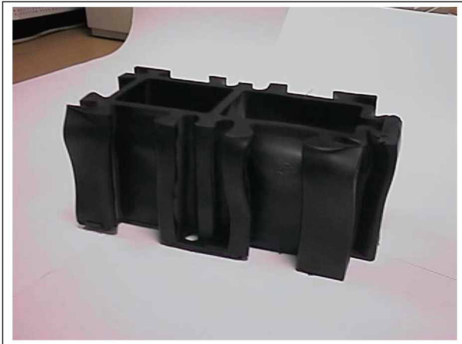
Figure 5: Experimental buckling failure mode of the Jig Brix.
