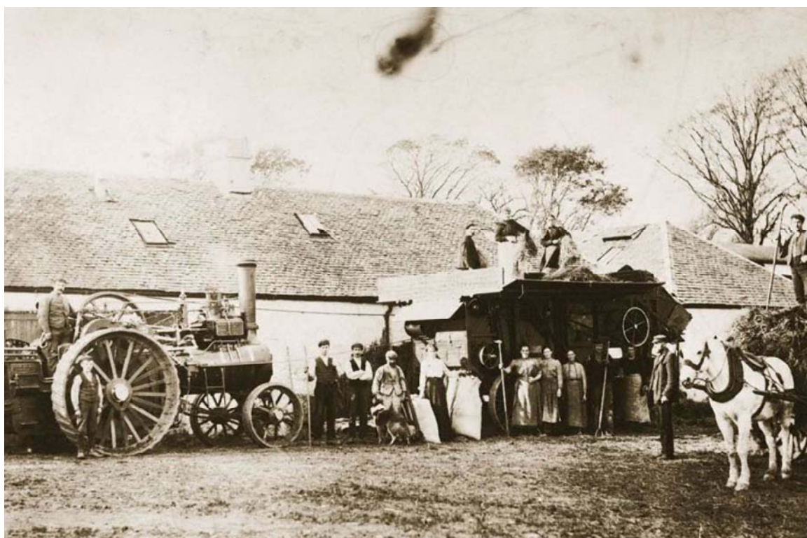
65. Steam threshing mill at Balgraystone Farm Newton Mearns, 1910. Source – copyright East Renfrewshire Council, licensor www.scran.ac.uk .
