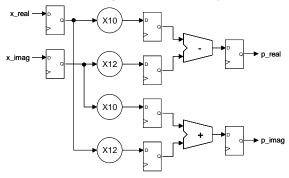
Figure 5. Circuit to multiply by 10+j12
