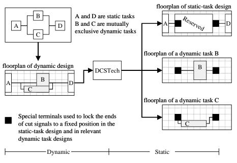
Figure 3: Floorplan of a DRL circuit containing two dynamic tasks before and after processing by DCSTech
