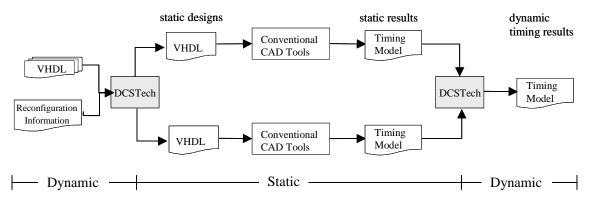
Figure 1: DCSTech: Domain conversion between static and dynamic domains
