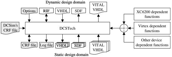
Figure 4: File flow for the extended DCSTech tool
