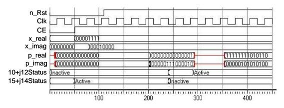
Figure 8. A backannotated timing simulation waveform for the dynamically reconfigurable complex multiplier
