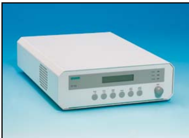
Figure 6.1 Photograph of the Linkam TP 93 temperature controller used in the experiments ( courtesy of Linkam Scientific Instruments, Ltd. )
