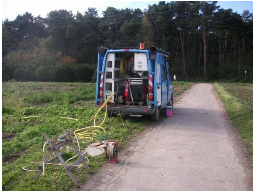
Figure 4.2. Erftverband custom built groundwater sampling vehicle; including submersible pumps, petrol generator and wet laboratory.
