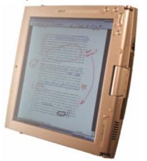
Figure 4: Acer TravelMate 100 running Microsoft Windows XP Tablet PC Edition and Internet Explorer with Callisto plugin. and folds back to cover the keyboard, thus allowing it to mimic the form-factor of a writing pad. Users interact with the Tablet PC with a stylus, which can be used to control the cursor and to draw and write directly on the screen.
