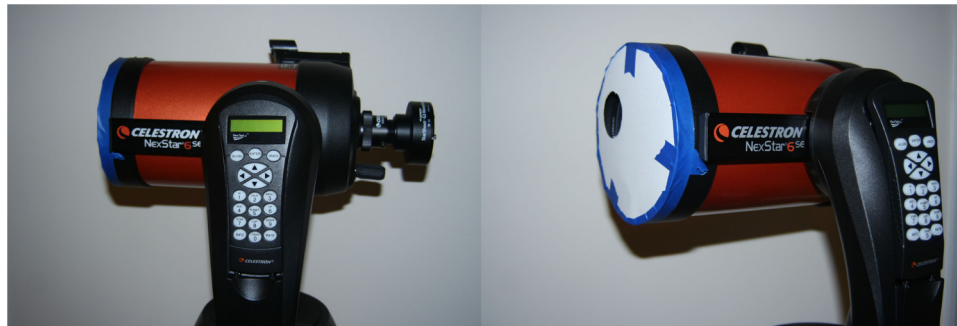
Fig. 11 Experimental sensor setup consists of a Celestron® NexStar® 6SE 1.5 m focal length telescope with a mask to reduce the aperture to 5 cm, and an Orion® Starshoot™ G3 monochrome camera.
