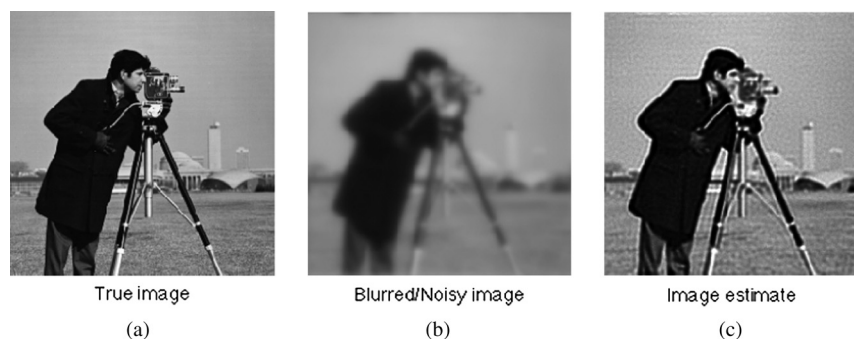
Fig. 6 In this demonstration, the true image (a) is blurred with an average short-exposure OTF with an r_0 of 2.6 cm. The blurred/noisy image (b) is the summation of 30 individual frames with independent realizations of Poisson noise. The image estimate (c) was obtained using the best estimate of r_0 = 2.6 cm with the cap on the number of iterations set to 5000.
