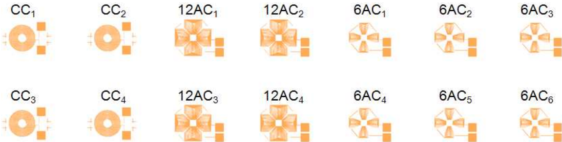
Figure D.2: Coil Referencing Scheme. With the Single Concentric Coils on the left, the numbering scheme is as above. (CC \rightarrow Single Concentric; 12AC \rightarrow 12-Turn Angular; and 6AC \rightarrow 6-Turn Angular.)
