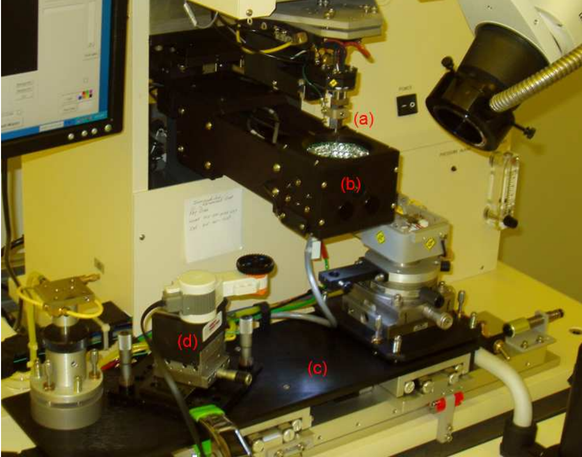
Figure 4.17: The Eagle 860 bonder was used to provide precise alignment of the coil and rotor. (a) marks the vertically adjustable head mount that will hold the inverted coil. (b) is an optical arm that provides imagery of both the head mount chip and the chip on the lower stage and allows for precise alignment of the two. It is retracted once alignment is achieved. (c) is the XY-adjustable stage where the custom rotary stage (d) sits.
