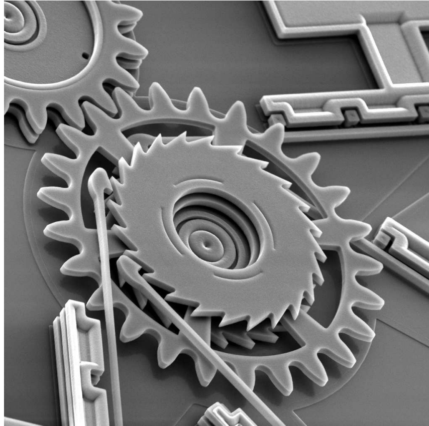
Figure 1.1: A complex MEMS ratchet system of gears created by Sandia National Labs [2].
