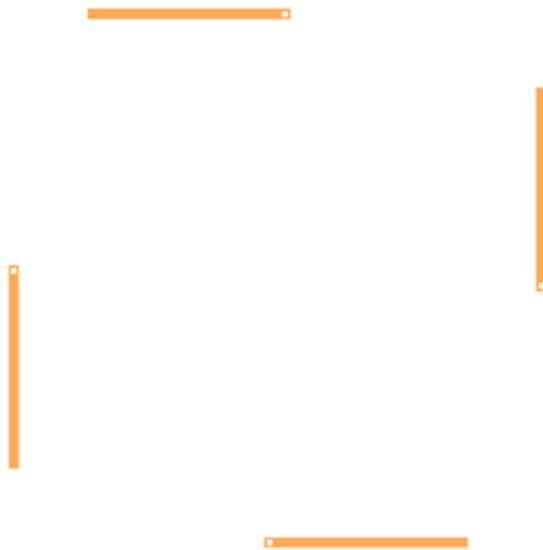
Figure B.6: Submask 3 - Zoomed in Nitride Etch Holes. Small holes were made into the nitride protective layer to provide vias between the coil and the runner.
