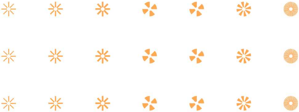
Figure B.8: Submask 5 - Magnet Nickel Plating Seed Etch. Pattern for etching the seed off of the rotor magnet slide. This mask was not used in this effort because the seed layer was not expected to significantly influence the output of the generator.
