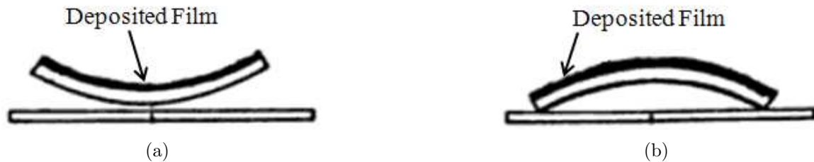
Figure 4.11: Diagram of tensile (a) and compressive (b) stresses on two layers with different coefficient's of thermal expansion [56].
