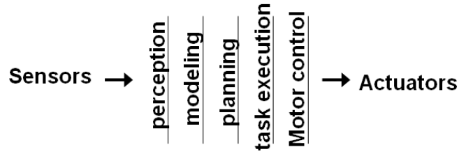
Figure 9. Traditional decomposition of mobile robot control system into functional modules [43]
