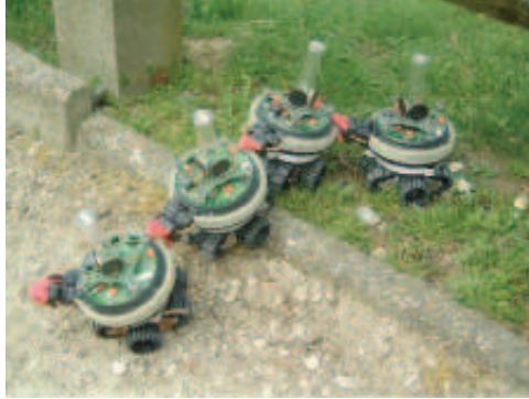
Figure 2.7: Swarm-Bot . - A swarm-Bot working together to navigate rough terrain [20].
