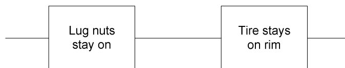
Figure 2.10 Example Reliability Block Diagram
