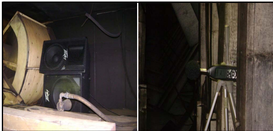
Figure 12: A: Speaker location at headgate drum and B: Sound meter on tripod
