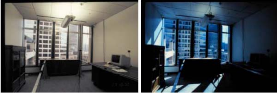
Figure B-2. Interior view of test room on a partly cloudy day. The EC windows are in the clear state at 10:30 under diffuse light conditions (left). When sun enters the window, the EC switches to its fully colored state by 10:50 (right) (Lee, et al., 2000).
