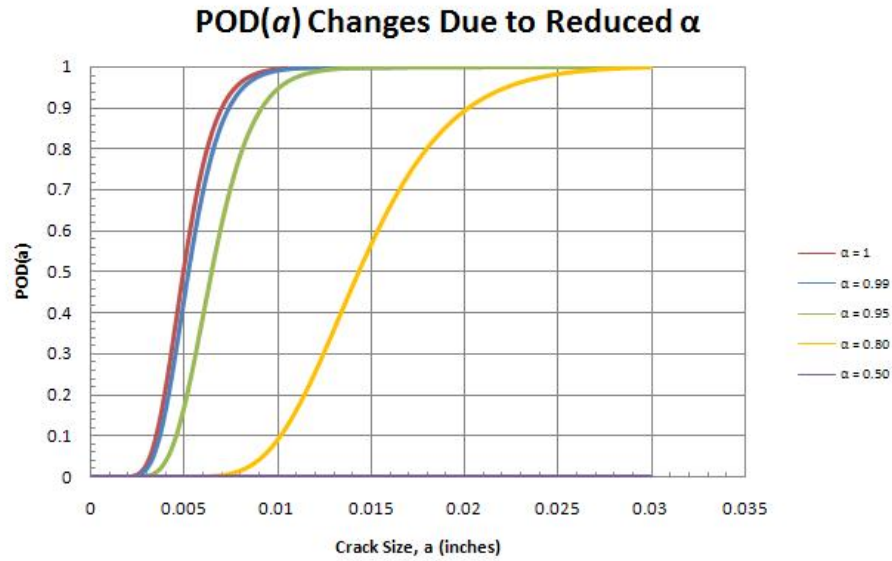
Figure 5.17: Decreasing \alpha_d “lowers” the regression line in Figure 5.1, reducing POD( a ) for all crack sizes
