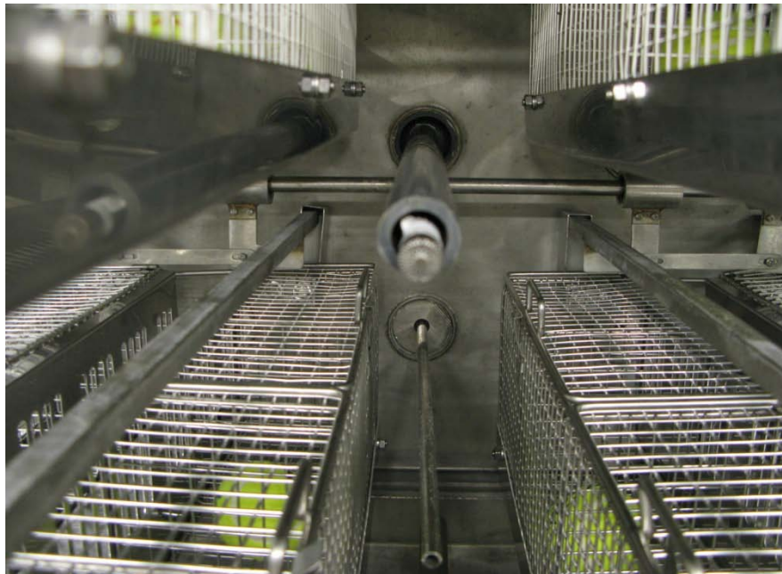
Figure 9. Microphone passed through PVC pipe to central reference point
