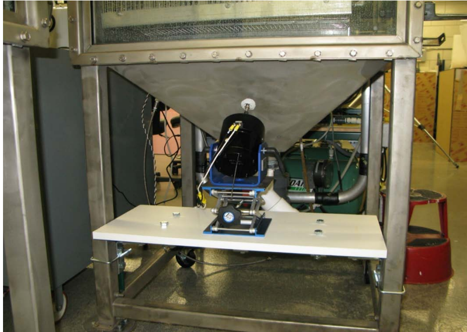
Figure 8. Shaker mounted on shelf between chamber legs
