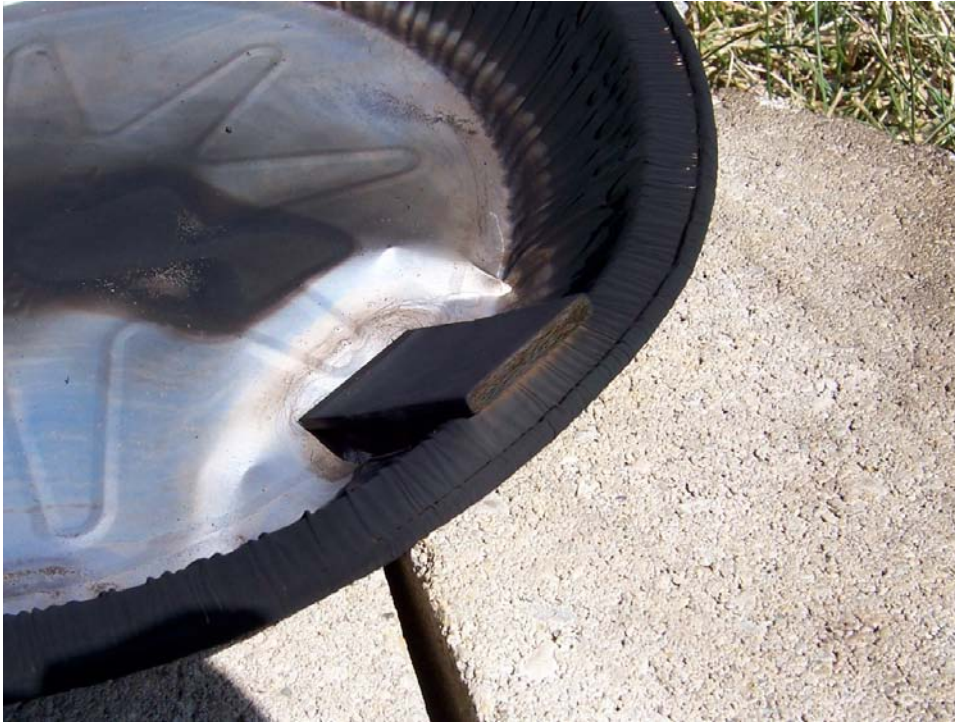
Figure 3 ACM ticket after burn with obvious signs of delamination
