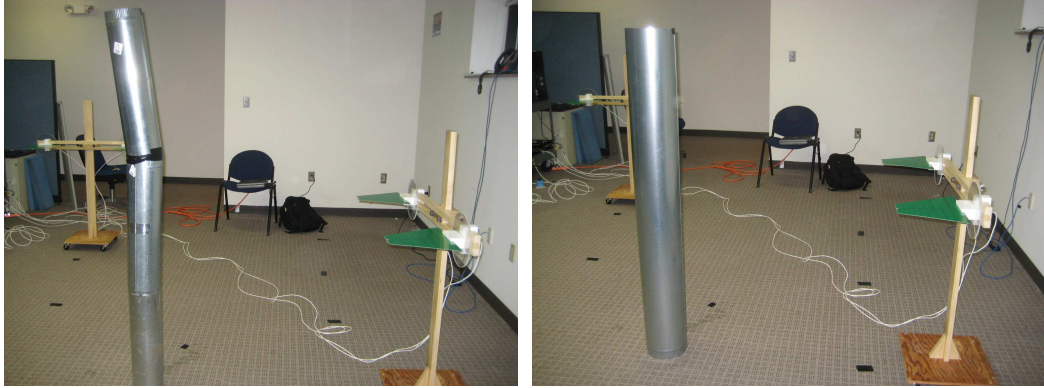
(a) 6 ft Tall by 6 in Diameter Metal Tube at 0° Rotation
