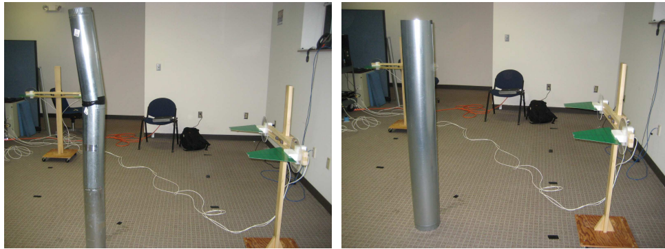
(a) 6 ft Tall by 6 in Diameter Metal Tube (b) 5 ft Tall by 8 in Diameter Metal Tube
