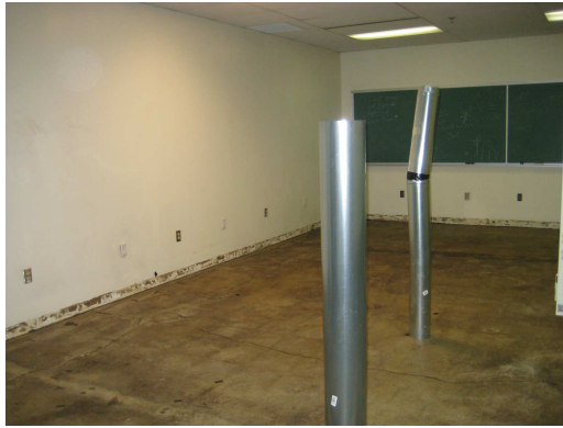
(b) Targets: 6 in Diameter Tube at (2.5 m, 2.7 m) and 8 in Diameter Tube at (4.1 m, 2.8 m)
