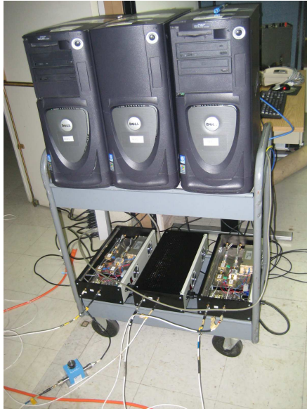
(a) Radar Systems 1, 2, and 3's Computers and Radar Boxes
