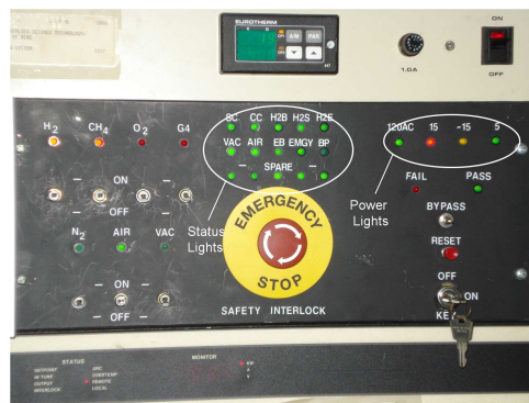
Figure 3.11: AFRL/RZ MPECVD system interlock panel.
