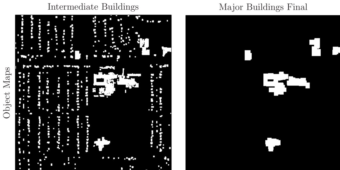
Figure 4.21: The intermediate “building” object map (left image) is morphologically opened with a 7 \times 7 SE, dilated with a 5 \times 5 SE, and then close with a 3 \times 3 SE to produce the “major buildings” final object map (right image). White pixels represent “major buildings” and black pixels represent “not major buildings areas”.
