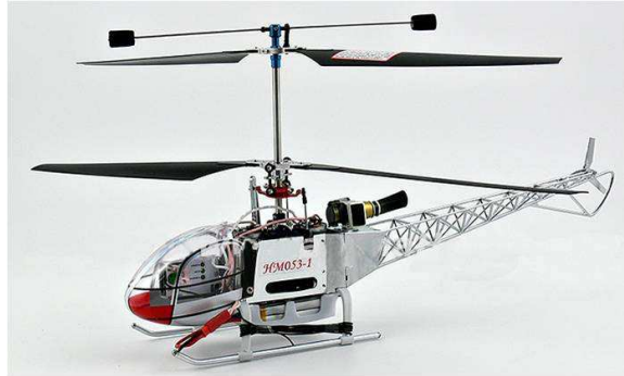
Figure 3.2: Walkera 53-1 (El Toro) . This commercially-available, remote-controlled, micro-sized helicopter is selected for modeling and autonomous control.
