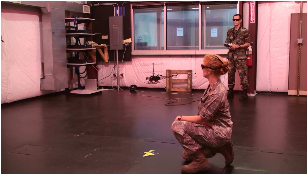
Figure 4.10: Hardware Test at the IFF. The IFF consists of a flight test room and a control room with a window separating the two. The LQR regulator is controlling El Toro while manually injecting disturbances.
