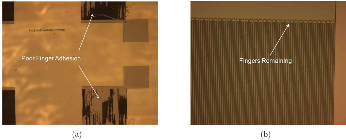
Figure B.34: Series 7 Quartz Lithography (a) Sample 7.1 after development on spinner. (b) Device 7.3.2 after development by immersion.
