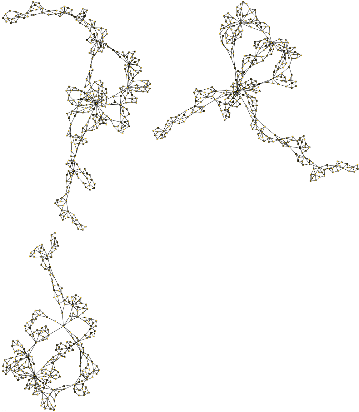
Figure A.5: Obfuscated Circuit Variant Graph after applying 1000 iterations, 3 replacement sizes, and FFTTT library generation option to circuit C17+C17+C17 . (943 gates, 155 levels)
