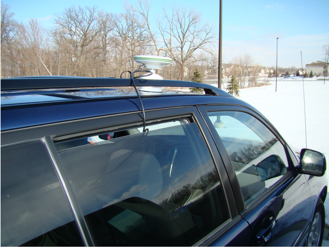
Figure 4.7: A magnet-mounted GPS antenna for the Leica GPS1200 Surveying System.
