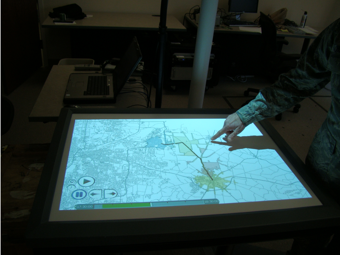
Figure 5.1: Pictured here is the MERL Diamond-Touch Table with World Wind 1.4 software. Vehicle tracklets and alpha hulls from our process are easy to view and manipulate collaboratively in this environment.
