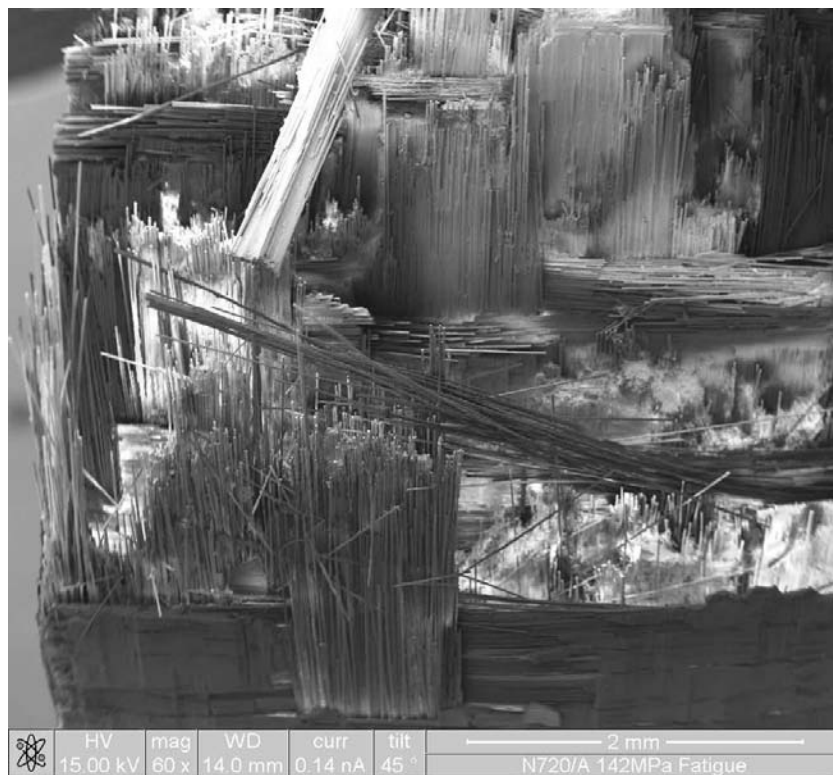
Figure 97. 142 MPa Fracture Surface, Rear Left Aft Looking Forward, 60x
