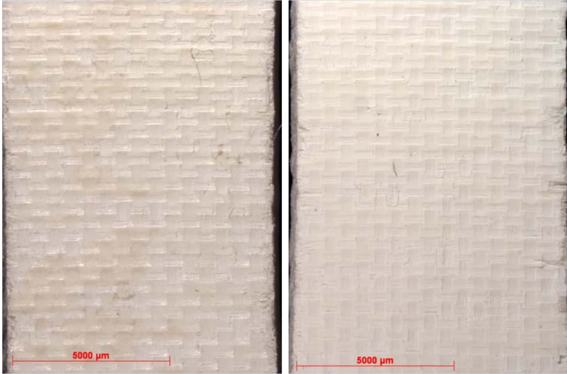
Figure 43. 121.5 MPa Specimen Pre and Post Test (Flame Side)
