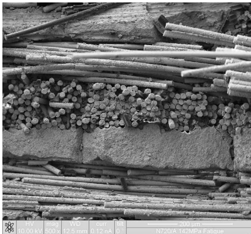
Figure 85. 142 MPa Fracture Surface, Front Right Fiber-Matrix, 500x
