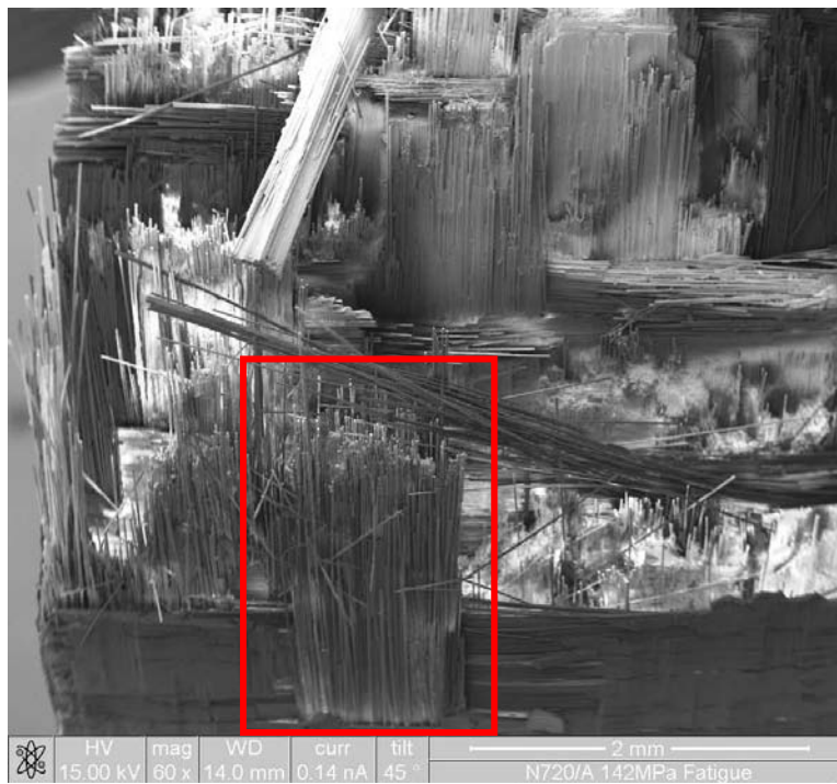
Figure 68. Rear Left Edge Fracture Surface (Flame Side Towards Top)
