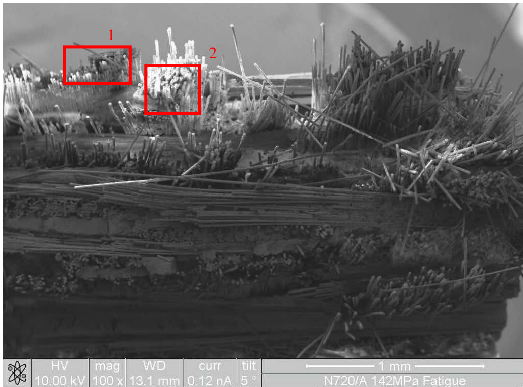
Figure 58. Front Right Edge Fracture Surface (Flame Side at Top)
