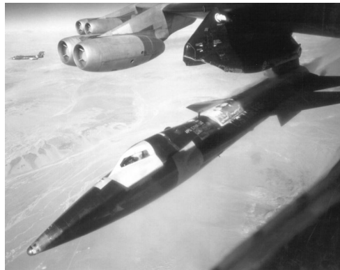
Figure 4. This photo, taken from a B-52, pictures the X-15 immediately after launch with an F-104 flying chase [7].
