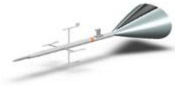
Figure 3. Nose-mounted Air-data Boom
